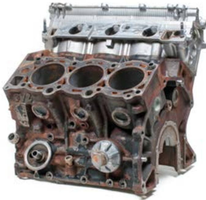
Figure 1 —Cylinder block with head attached
