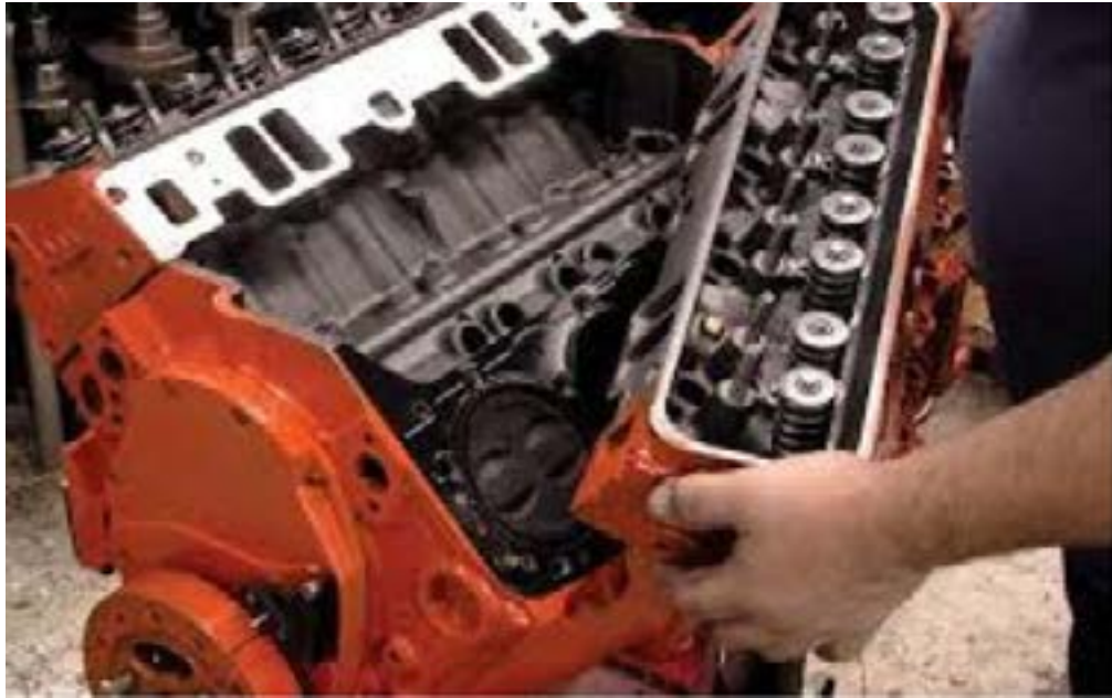
Figure 11 —Cylinder head being attached to engine block
