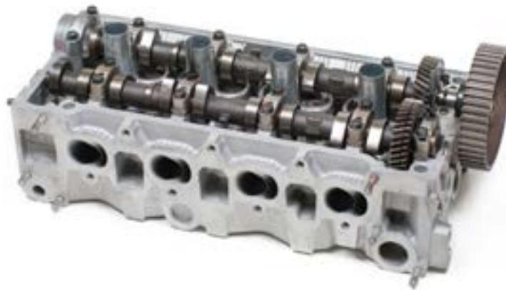
Figure 17 —Camshaft located over the head
