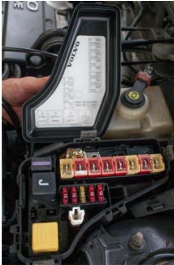
**Figure 6**—Typical fuel pump relay location
