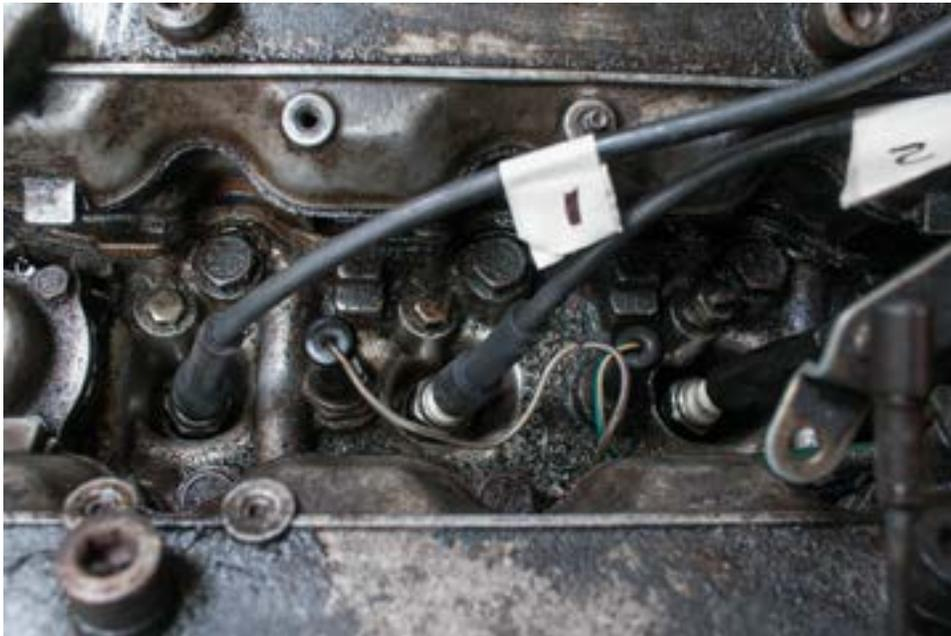
**Figure 5**—Spark plug wires attached to engine
